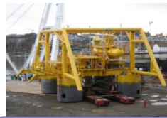
2007 Tordis Subsea water removal & injection, oil & gas boosting
