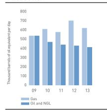
Total production from the SDFI portfolio was nine per cent lower than in 2012. The output of liquids (oil, NGL and condensate) declined by four per cent compared with the year before, while gas production was down by 12 per cent.
